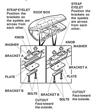
7. Fit bracket A over the threads of the bolt where it goes through the roof box. Install a washer over the threads, and loosely install a knob. Install a second bolt the same way. Install bracket A so that the right and left strap eyelets are positioned directly across from each other.
