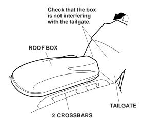
2. Open the roof box. Slide each plate forward or backward until the holes in the plate are over the front roof rack crossbar.
