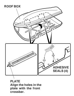
3. Attach adhesive seals over the unused rear mounting holes in the bottom of the roof box. The seals help prevent water from entering the roof box. Remove the roof box from the vehicle.
